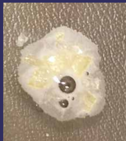
The oxidative degradation of the powder of polydiacylhydrazine. The bubble is nitrogen gas evolved during decomposition
