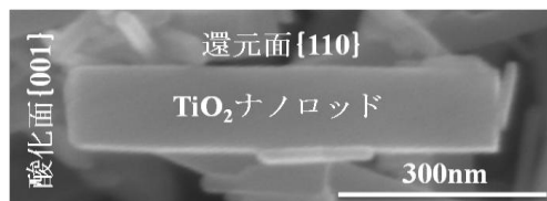
Fig.1 SEM image of TiO 2 nano-rod
