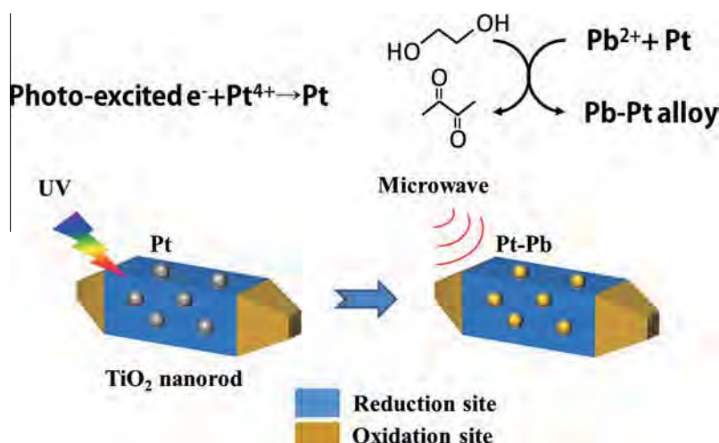
Scheme 1. Preparation procedure for site-selective Pt–Pb deposition on the reduction site of rutile TiO 2 nanorod (2-step method). Photoreduction of Pt 4+ on the reduction site of TiO 2 nanorod and followed by microwave assisted polyol reduction of Pb 2+ and simultaneously alloying with Pt.
