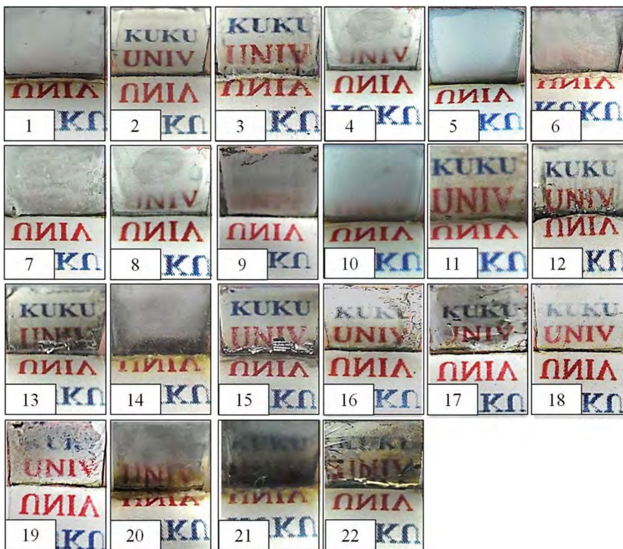
Fig. 4. Micrographs of the Al films obtained by the electrodeposition of Al from the EMIC/ \text{AlCl}_3 (EMIC: \text{AlCl}_3 = 1:2 (molar ratio))/toluene (9.25 M) baths containing (1) non-additive, (2) 4-PCAH, (3) 3-PCAH, (4) 2-PCAH, (5) 4-PCA, (6) 3-PCA, (7) 2-PCA, (8) 4-MP, (9) 3-MP, (10) 2-MP, (11) 4-AP, (12) 3-AP, (13) 2-AP, (14) BH, (15) P-4-CA, (16) P-3-CA, (17) P-2-CA, (18) AH, (19) AA, (20) 4-PH, (21) 4-AP and (22) PY. Deposition time: 2 h; constant current density: 8.0 \text{ mAcm}^{-2} ; and additive concentration: 1.8 mM. The characters “KUKU UNIV” were reflected on the deposited Al films (upper part: Al film, lower part: printed-out characters).
